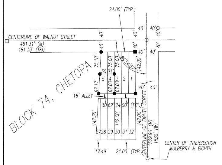
A BOUNDARY SURVEY WAS CONDUCTED FEBRUARY 8, 2022 FOR WOOD—DULOHERY REAL ESTATE TO ESTABLISH THE BOUNDARIES OF THE TRACTS DESCRIBED BELOW AS SHOWN ABOVE. REFERENCE WAS MADE TO THE ADDITION PLAT, RECORD DEEDS, A 2006 SURVEY BY TRI—STATE ENGINEERING AND A 2003 SURVEY BY WHITE IN BLOCK 21. SURVEY MONUMENTS WERE FOUND AND SET AS SHOWN ABOVE. THE TRACTS MAY BE DESCRIBED AS:
